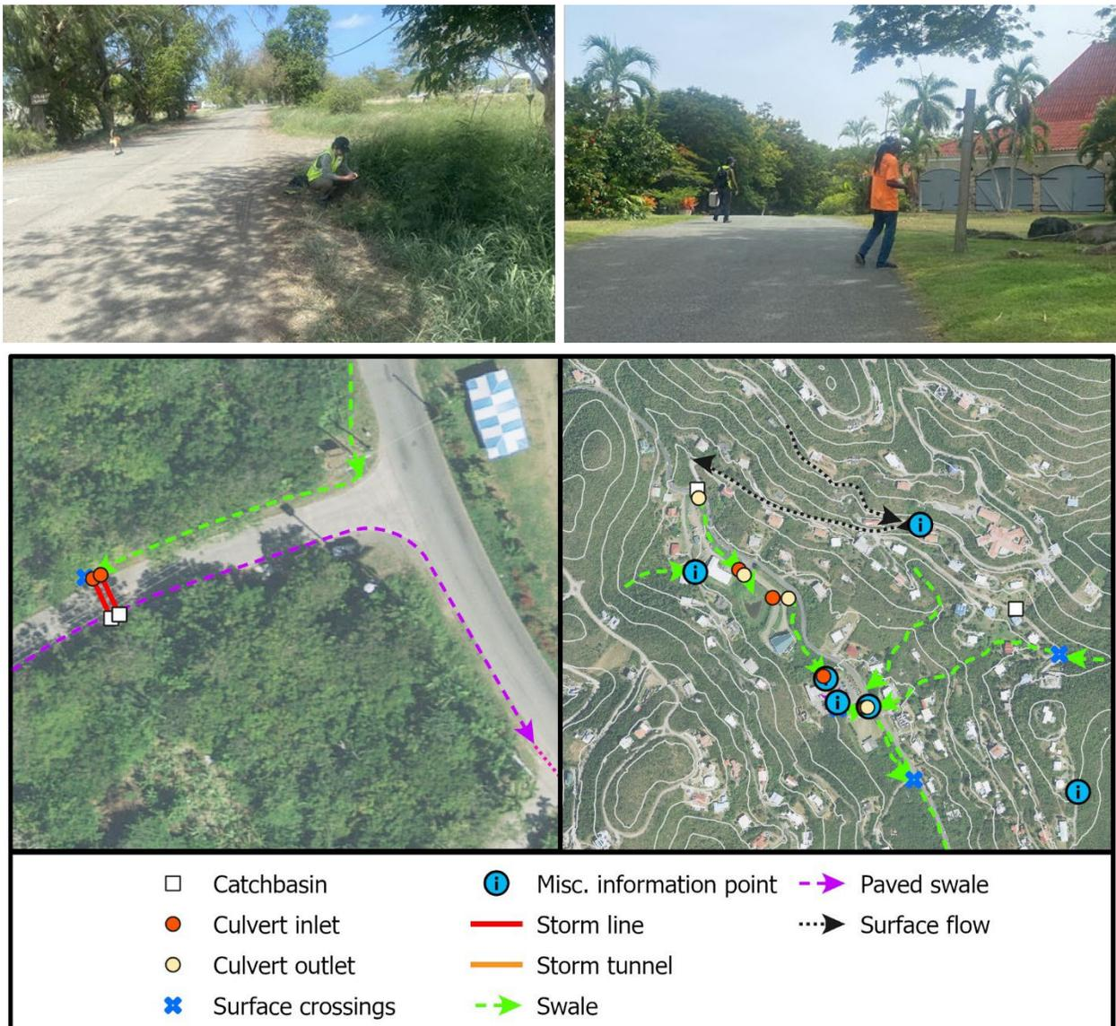
Figure 45. Inspection of existing stormwater infrastructure during field assessments (above) and an example of the maps produced (below).
